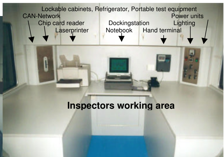
Pic 27: The Inspectors work place with PC area including docking station and Printer
